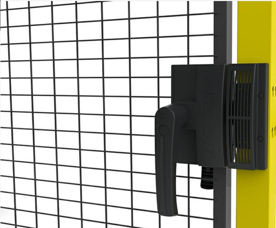
The X-Guard Hitch Lock is a reliable locking system for machine guarding, offering a secure alternative to the X-Lock. Designed for precision and safety, it features an adjustable hitch to eliminate internal play and ensure a firm closure. The integrated mounting allows for easy installation of non-contact switches for optimal safety.
