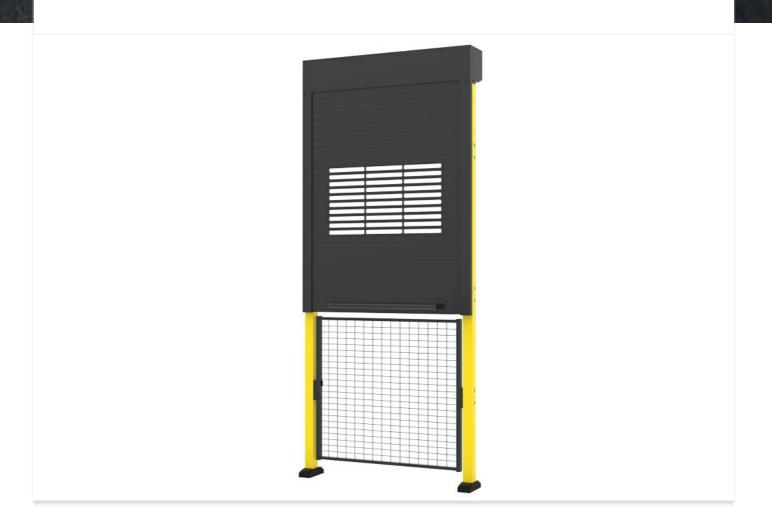
The manual roller door consists of a modular system with integrated spring loaded shaft and is available as standard in three widths and two heights. X-Roll-up wraps the aluminium rolling door during opening onto a shaft in the box at the top.
