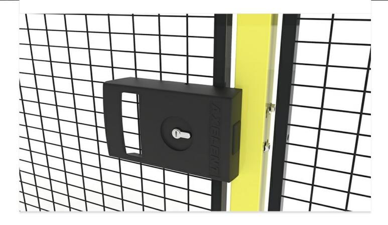
The lock has a unique design that requires no additional lock housing, just add a standard cylinder such as Euro. The lock is robust with a cover in metal to withstand tough conditions, and is tested and approved according to SS-EN 12209:2016. X-It fits both hinge or sliding doors. The lock can also be combined with a mechanical panic / emergency unit. The product is patent pending.
