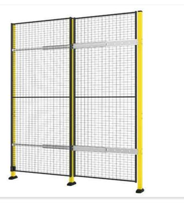
The X-Guard single sliding door without rail is designed for industrial environments where overhead clearance is essential. Unlike traditional sliding doors, it operates without an upper rail, making it the ideal choice for areas where forklifts or overhead cranes need unrestricted access. Available in multiple widths—900mm, 1400mm, and 2900mm— and with a maximum height of 2500mm, this door provides a practical and efficient safety solution.
