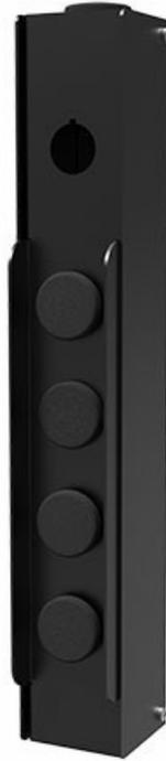
The X-Guard push button enclosure is a robust and adaptable solution for integrating push button controls into sliding door locking systems. Made from black powder-coated metal (RAL 9011), it accommodates up to 4 push buttons ( $\varnothing 22.5$  mm) and 1 emergency stop button, offering a streamlined way to manage access in machine guarding applications.
