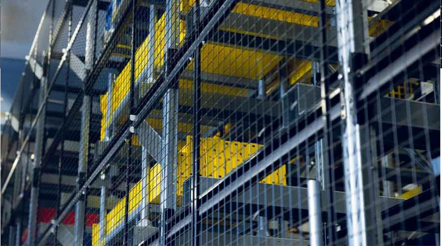
Post extensions are available as an accessory. This makes it possible to mount the anti-tip protection higher than the post itself.
