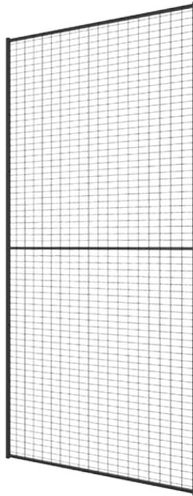
The size of mesh is cc 50x30 mm. The mesh consists of vertical wires of Ø 3 mm and horizontal wires of Ø 2.5 mm. The recommended safety distance is 200 mm.
