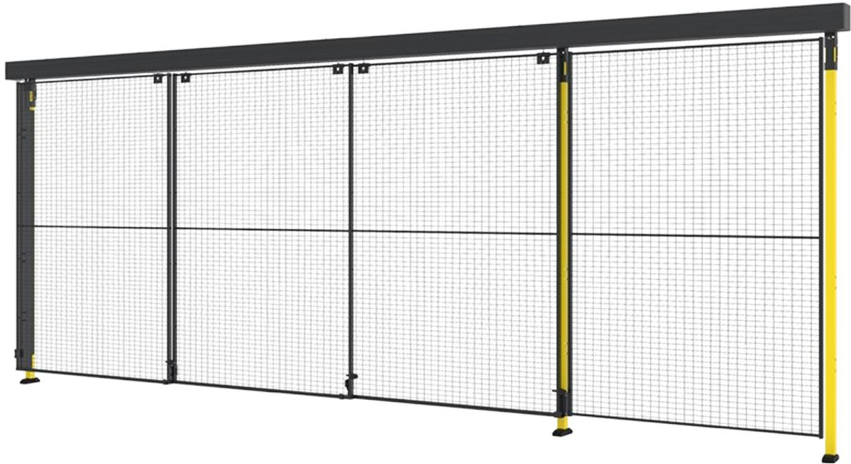
The X-Guard triple telescopic sliding door is designed for industrial settings that require a large opening but have limited space for traditional sliding doors. Featuring a 3-step rail system, the panels overlap instead of sliding fully outward, reducing the need for side clearance while maintaining easy access. With a maximum width of 3x1500 mm and a height of 2500 mm, it offers a practical and efficient safety solution.
