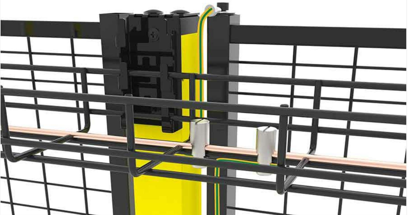
The kit is comprised of a “plug-and-play” connector for the posts and the panels, which are preassembled with a tightening screw and a connecting wire. The connector for the posts is slid through one of the key holes, the connector for the panels is slid into one of the vertical frame tubes from top or bottom. After tightening, good connection is achieved. Application of the kit has been successfully tested to IEC 61537, section 11.1.2 by an independent certification institute.
