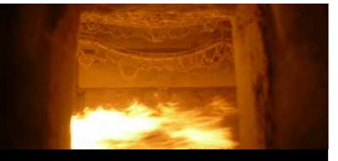
In the bottom of the oven are four large oil burners used to create the fire. The fire rages for 90 minutes, at the end of which the temperature reaches almost 1000° Celsius.
