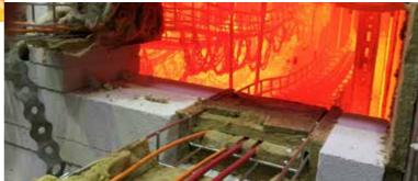
When a cable short-circuits (the breaker trips) it counts as eliminated. Because the cable was previously approved in another type of test it is now the wire tray's fire resistant properties that decide how long the cable will hold out.
